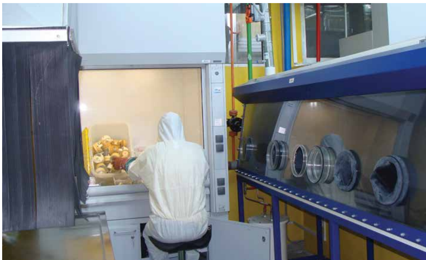
Removal of sources from ionization fire alarm detectors in the Reception and Preparation Laboratory Complex in Specialised Division Permanent Repository for Radioactive Waste – Novi Han, Photo SE RAW
